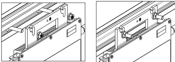
**Step 4. Connect the APsystems Microinverter cables to the AC bus cable.**
