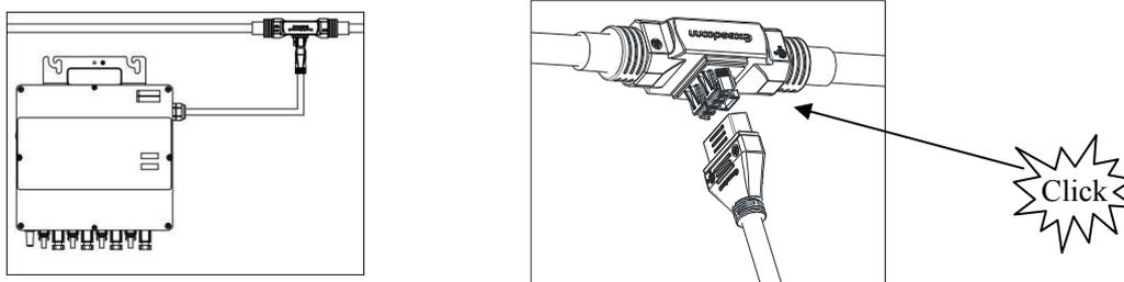
*NOTE: AC connector interface as follows, from left to right PE, N, L3, L2, L1.*
